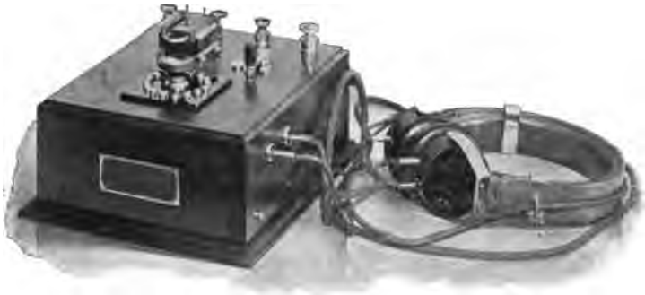
FIG. 11.—MICROPHONE WITH TELEPHONE RECEIVERS CONNECTED.
